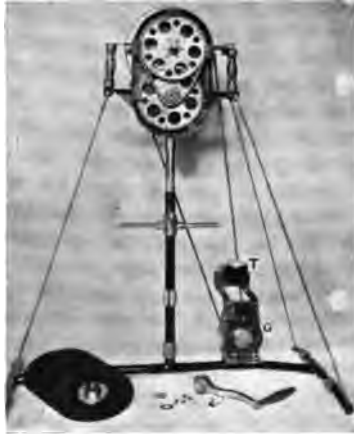
FIG. 157 a .—Generating plant of knapsack set (assembled).
